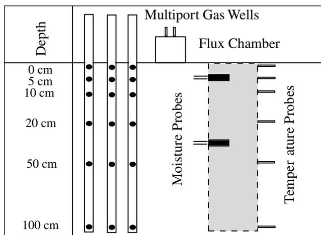
**Figure 1.** Site setup: Subsurface instrumentation and CO<sub>2</sub> sampling. Wells are located 1 m apart.
