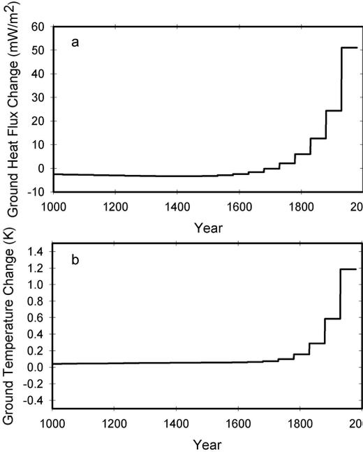
Figure 1: Heat flux (a) and Ground temperature (b) Histories in Canada inferred from geothermal data. One hundred and twelve temperature logs were used in calculation. Standard error of the model parameters are included within the lines shown.
