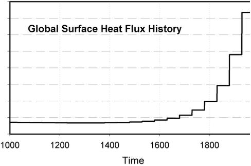
Figure 2: Global Heat Flux History inferred from geothermal data. Six hundred and sixteen temperature logs were used to calculate this average. Standard error of the model parameters are included within the line shown.
